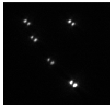
Fig. 446 Double lobed PSF created by a double phase-ramp in the pupil plane
